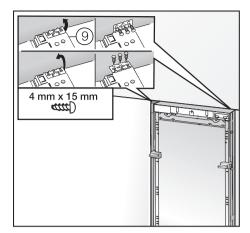
Pull out the lugs for the side fixing plates (9).
